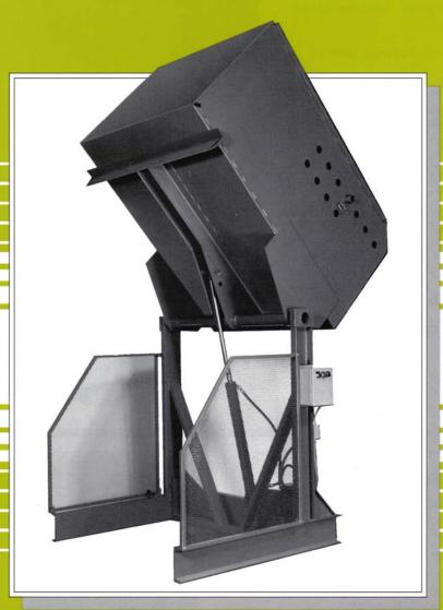
Our container dumper provides a cost-effective, safe and ergonomic way of dumping materials out of boxes, gaylords, carts or hoppers. The PD25 series of dumpers has a capacity of 2,500 pounds and a dumping height of up to 70". This heavy-duty, low-cost machine can be modified to dump most any width container.
