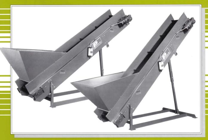
Our AL Series of incline, cleated, belt conveyors are designed to convey any product or material. The standard units are equipped with 1/2 HP motor and drive making them ideal for feeding granulators, crushers, shredders or all types of containers. These conveyors also have adjustable legs as a standard feature which gives them multiple use capabilities. These machines can be adjusted in 1" increments from 25 degrees to 45 degrees.
